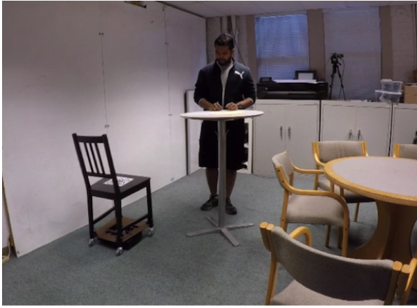
Fig. 4. Example of participant yielding to the ChairBot, robot begins at bottom-left of frame and stops when it reaches the file cabinets.
